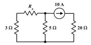
What value of  $R_x$  will absorb maximum power from the remainder of the circuit?
